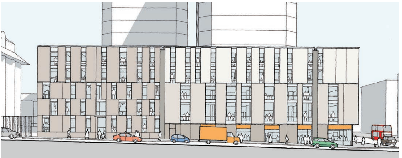
Articulation, scale and function: horizontal vs. vertical, sandwich vs. townhouse terrace, module and tone related to brief
